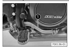
The footbrake pedal **1** is located in front of the right footrest. The footbrake pedal operates the rear brake.
