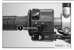
The flasher switch • is fitted on the left side of the handlebar.
