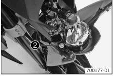
Adjust the beam distance of the headlight by turning screw ②.
