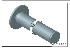
Move the handlebar to the straight-ahead position. Move the throttle grip backwards and forwards to ascertain the play in the gas Bowden cable.
