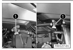
The fuel taps • are located on the left/right under the fuel tank.
