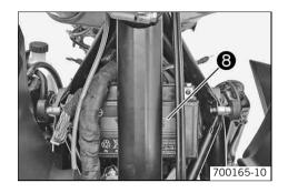
Pull battery 3 up and out of the battery rack. Take the battery out of the frame toward the right.
