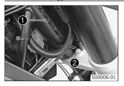
The chassis number **1** is stamped on the right of the steering head. The type label **2** is on the right of the frame behind the steering head.
