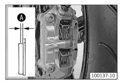
Check the brake linings for minimum thickness •.
