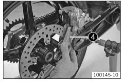
Pull the rear wheel and brake caliper support 4 together to the rear until you can swing the brake caliper support to the side.
