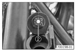
Turn the adjusting wheel until the desired digit is next to marking ②.
