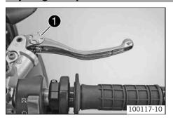
Adjust the basic setting of the handbrake lever to your hand size by turning adjusting wheel 1.
