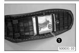
You can find the owner's manual 1 in its protective case on the underside of the seat.
