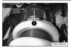
The shock absorber part number  $oldsymbol{0}$  is stamped on the top of the shock absorber above the adjusting ring toward the rear.
