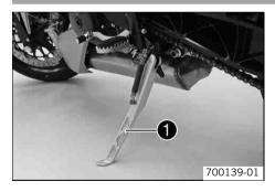
The side stand lacktriangle is coupled with the safety electric starter system - see the riding instructions.
