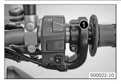
The emergency OFF switch **1** is fitted on the left side of the handlebar.
