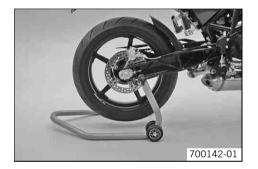
Insert the work stand adapter in the work stand and screw it into the link forks.
