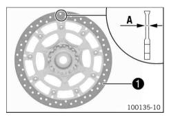
Check the thickness of the front and rear brake discs in several places to ensure that it conforms to measurement .
