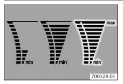
The temperature display consists of 12 bars. The more bars showing, the hotter the coolant. When the top bar lights up, all bars begin to flash and the temperature warning light starts to show.
