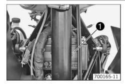
Push battery ● from the right into the frame. Position the battery in the battery rack.
