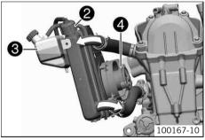
The coolant is cooled by the air stream and a radiator fan  $oldsymbol{0}$ , which is controlled by a thermoswitch.
