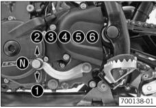
The gear positions can be seen in the photograph. The neutral or idle position is between the first and second gears. CONTROLS 37
