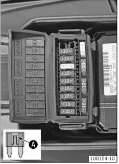
Remove the defective fuse.
