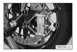
Clean and grease the thread of the wheel spindle and screw 1.
