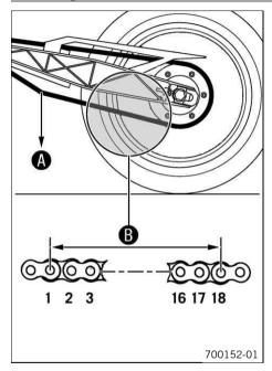
Shift into neutral, and pull the lower chain section with the specified weight .
