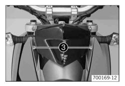
Position the headlight mask. Mount and tighten screws 3.
