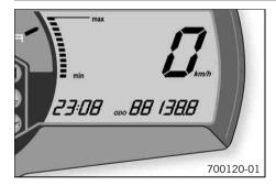
In the **QDO** display mode, the total distance traveled is shown in kilometers or miles.
