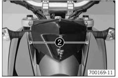
Position the headlight mask. Mount and tighten screws ②.
