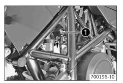
Pull the Map-Select switch with holder 1 downward off of the retaining bracket.
