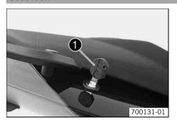
The seat lock **①** is located to the right of the seat. You can lock it with the ignition key.
